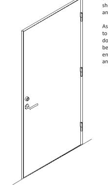
Clearance between the door and frame, when fully assembled, shall not exceed 3mm horizontally/2mm vertically. The space between the frame and the wall should be compacted hard and accurately with non-flammable insulation material. Minimum 92mm measured from the hanging side. Where an acoustic insulating door is concerned, it should be sealed on at least 1 side (hanging side) when door  $\leq$  Rw33, and on 2 sides when door  $\geq$  Rw38.
